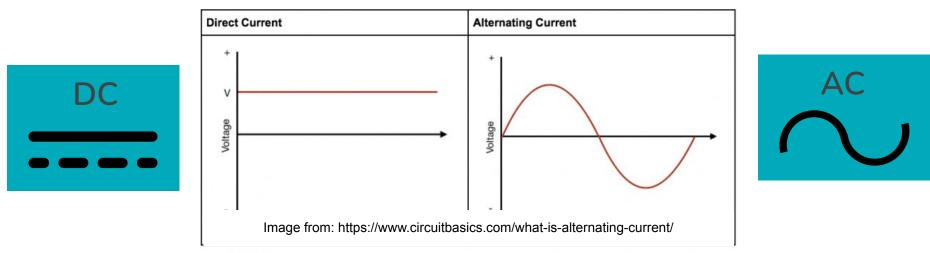
PV Modules generate direct current (DC), which is then changed into alternating current (AC) inside the inverter, which is the type that is used for most of our loads.
