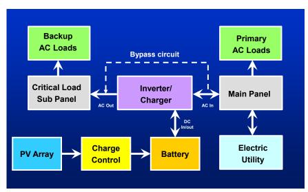
Figure 25. Utility-interactive systems with battery storage are similar to uninterruptible power supplies, and have many similar components.
