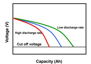
Figure 27. Battery capacity is a measure of the stored energy that a battery can deliver under specified conditions.
