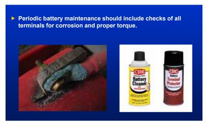
Figure 115. Periodic battery maintenance should include checks of all terminals for corrosion and proper torque.
