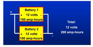
Figure 31. Parallel battery connections increase capacity.
