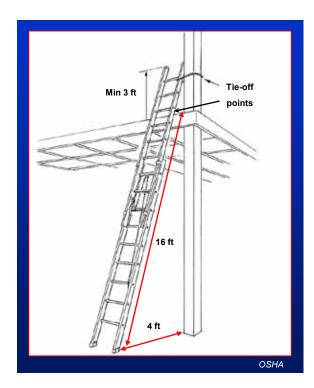
If using ladders where the employee or the ladder could contact exposed energized electrical equipment, such as transformers or overhead services, ladders must have nonconductive side rails such as wood or fiberglass. Face the ladder when going up or down, and use at least one hand to grab the ladder when going up or down. Do not carry any object or load that could cause you to lose balance while climbing ladders.
