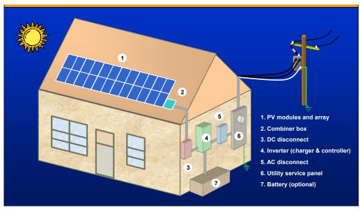
Figure 1. - PV system components
