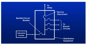
Figure 101. Many small residential and commercial PV systems can be interconnected by adding backfed circuit breakers to distribution panels as long as certain conditions are met.
