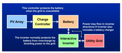
Figure 39. Battery-based interactive inverters operate as diversionary charge controllers to regulate battery state-of-charge.
