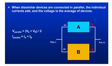
Figure 65. Dissimilar current PV modules and strings having similar voltage may be connected in parallel.
