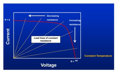
Figure 52. The specific operating point on an I-V curve is determined by the electrical load resistance according to Ohm's Law.
