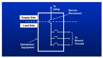
Figure 100. Interactive inverters may be connected to either the load side or the supply side of the service disconnecting means.
