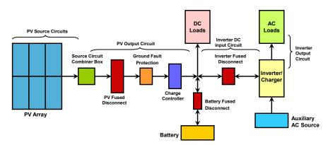
Figure 81. For stand-alone PV systems the PV array charges the battery, and the battery provides dc power to the inverter which can produce ac power output at any time.
