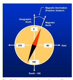
Figure 11. Magnetic compass readings must be corrected for magnetic declination.
