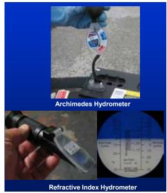
Figure 117. Hydrometers measure electrolyte specific gravity (SG).
