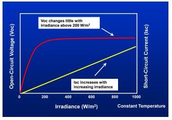
Figure 53. Changes in solar radiation have a direct linear and proportional effect on the current and maximum power output of a PV module or array.
