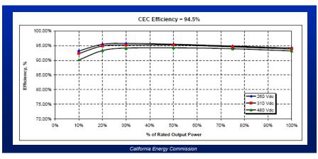
Figure 78. Inverter efficiency testing is conducted over a range of operating voltages and power levels.
