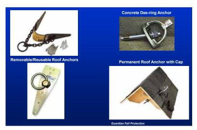
Figure 88. Safety line anchorages must be independent of any platform anchorage and capable of supporting at least 5,000 pounds per worker.
