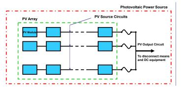
Figure 79. The PV power source consists of the complete PV array dc power generating unit, including PV source circuits, PV output circuits, and overcurrent protection devices as required.
