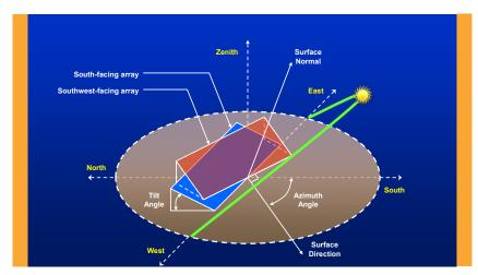
Figure 13. The orientation of PV arrays is defined by the surface azimuth and tilt angles.
