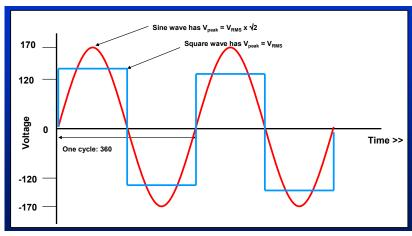
Figure 76. Sine waves, square waves and modified square waves are examples of common inverter ac waveforms.
