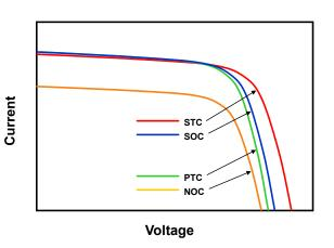
Figure 57. The differences between rating conditions can be clearly shown by the I-V curves.
