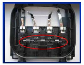
Figure 68. Bypass diodes are often located in module junction
