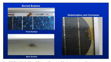
Figure 110. PV modules should be carefully inspected for any signs of discoloration, corrosion or delamination.
