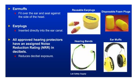
Figure 94. Hearing protection should be used whenever using machinery or power tools with noise levels exceeding 85 dB.
