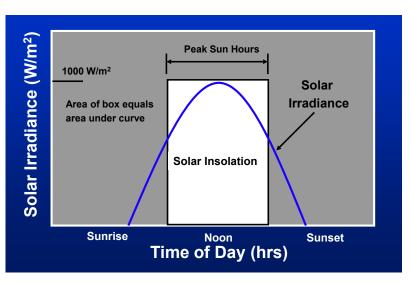
Figure 47. Peak sun hours (PSH) represents the average daily amount of solar energy received on a surface, and equivalent to the number of hours that the solar irradiance would be at a peak level of 1 kW/m².
