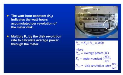
Figure 113. A standard watt-hour meter can be used to measure average power over brief intervals.
