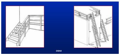
Figure 89. A stairway or ladder is required at points of access to a construction site where there is a break in elevation of 19 inches or more.
