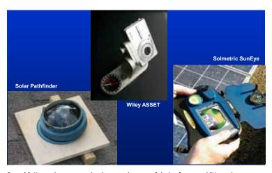
Figure 18. Various devices are used to determine the extent of shading for potential PV array locations.
