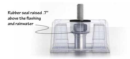
Our patented QBlock technology encloses the EPDM rubber seal – the ultimate barrier between the rafter and the rain – inside a cast-aluminum block and raises it <sup>7</sup>/<sub>10</sub> of an inch above the flashing where the rainwater flows. **This** completely protects the rubber seal from the elements for the life of the solar array.
