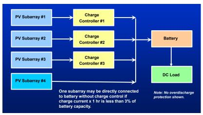
Figure 37. Multiple charge controllers may be used on individual subarrays for larger systems.
