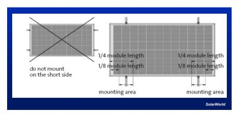
Figure 108. PV module specifications give the maximum mechanical loads that the module can support using specified supports and attachments.
