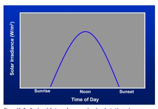
Figure 45. For fixed south-facing surfaces on a clear day, the incident solar irradiance varies in a bell-shaped curve, peaking at solar noon.
