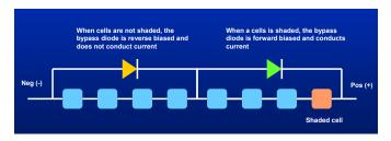
Figure 67. Bypass diodes are connected in parallel with series strings of cells to prevent cell overheating when cells or parts of an array are shaded.
