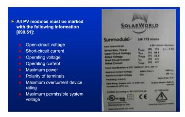
Figure 59. PV module nameplate electrical ratings govern the circuit design and application limits for the product.
