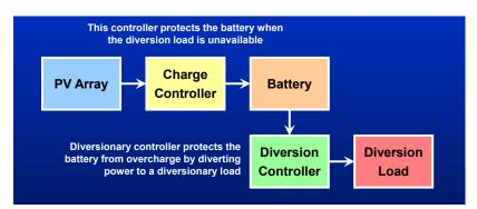
Figure 38. A diversionary charge controller diverts excess PV array power to auxiliary loads.
