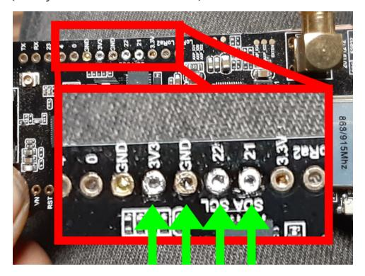
Insert the 4 pins that came with into those holes and solder them to the board:
