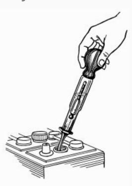
Measures the specific gravity in flooded lead-acid batteries
