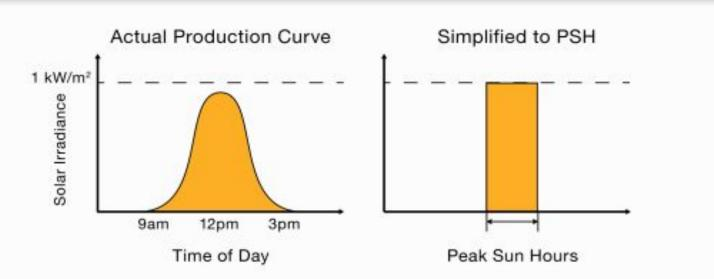
PSH makes it possible to estimate the size requirements of the solar array and the available solar window
