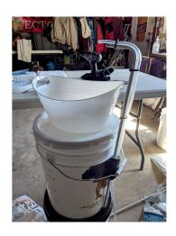
Now secure the tubing to the curtain rod with zip ties (making sure not to pinch the tubing too much). Carefully bend the curtain rod down slightly to ensure the water pours into the center of the wash basin.
