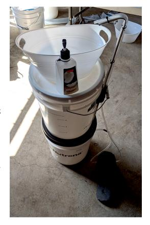
Take off the top bucket and remove the foot pump tube from the bottom bucket.
